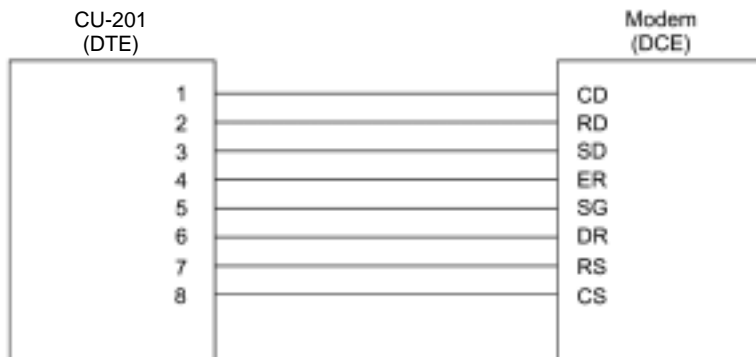
Cable Connection between CU-201 and Modem
